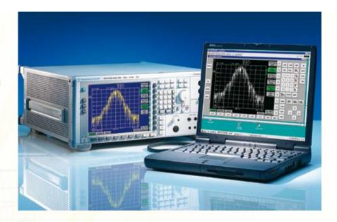
The low displayed average noise level of typ. –148 dBm in a 1 Hz bandwidth at 26 GHz, and –138 dBm (1 Hz) at 46 GHz, supports accurate and sensitive measurements.
